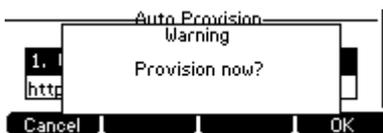
8. The handset will request its own software and configuration files. The device may power cycle whilst installing software and processing its configuration. If successful, the line provisioned will register for service
