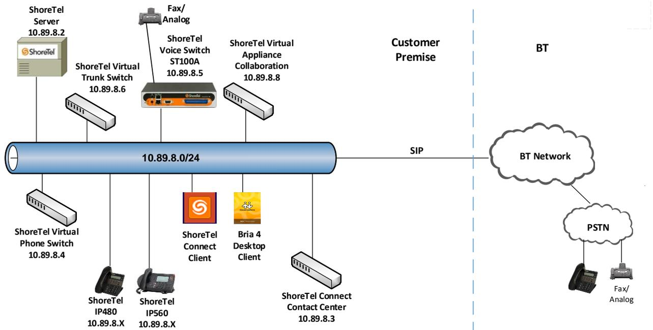
Figure 1: SIP Trunk Lab Reference Network
