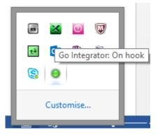
The icon should be green (or red when on an active call) if the User is successfully logged in. If this is not the case please check the Username, Password and Add-On Feature Package on the Business Portal match that has been entered into the application.
