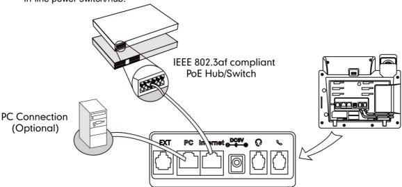
Note: If in-line power switch/hub is provided, you don't need to connect the phone to the power adapter. Make sure the switch/hub is PoE-compliant. The phone can also share the network with another network device such as a PC (personal computer). It is an optional connection. Important! Do not unplug or remove power to the phone while it is updating firmware and configurations.
