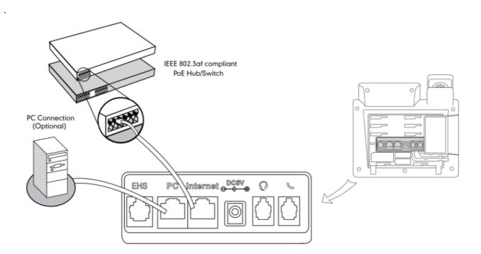
Please note that if an in-line power switch/hub is provided, you don't need to connect the phone to the power adapter. Make sure the switch/hub is PoE-compliant. The phone can also share the network with another network device such as a PC (personal computer). It is an optional connection.
