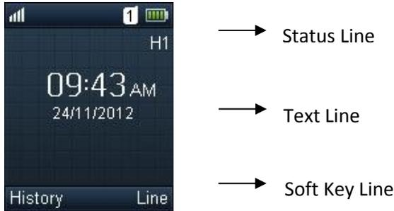
The LCD screen is divided into three parts: status line, text line and soft key line
