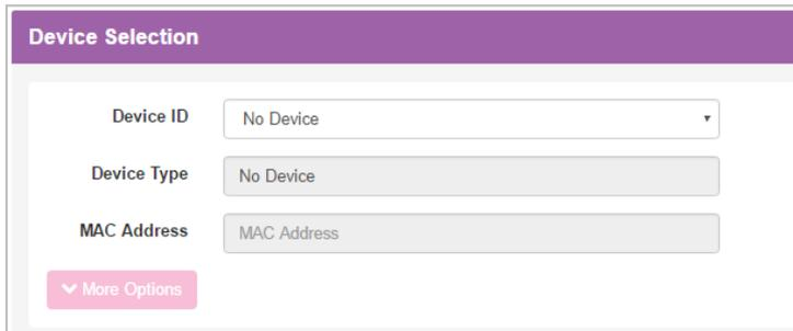
If you are using the Additional Line feature, whereby you want to add another line to an existing User's phone, then ensure you select that existing device. If you select **New Device**, you must choose the appropriate device type from the Device Type field and fill in the MAC Address (required).
