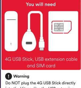
into the Hitron. Use the USB extension cable and keep at least 20cm away.
